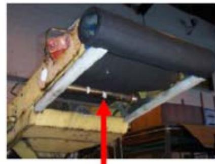
Figure 5 - Roller located under the conveyor belt
