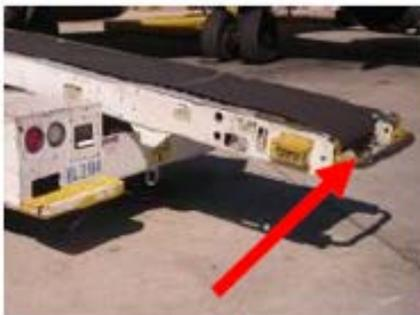
Figure 2 - Space between belt and spacer
