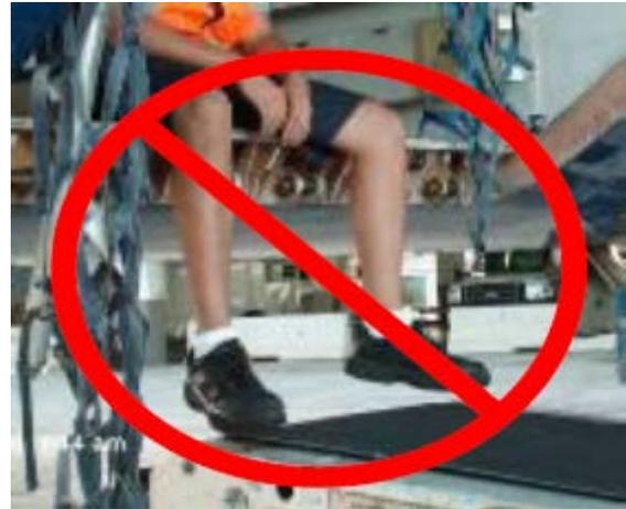
Figure 7 – Individuals should not sit on the cargo bin floor with their legs dangling out of the aircraft
