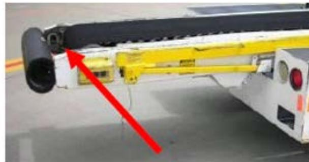
Figure 3 - Space between belt and spacer
