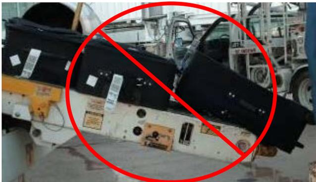
Figure 1 – Improper spacing of baggage
