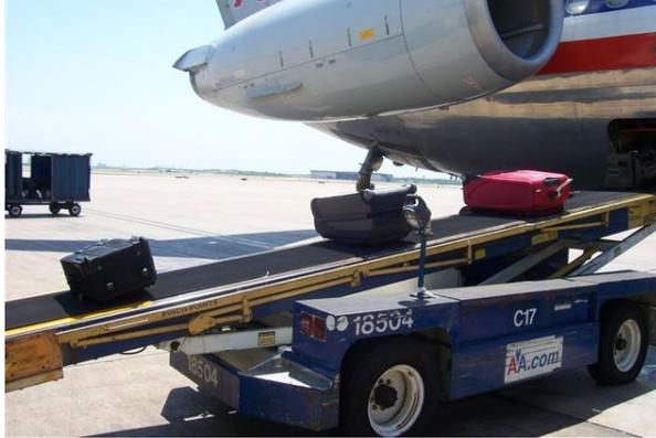
Figure 3 – Proper spacing of bags
