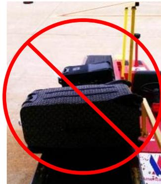
Figure 2 –Baggage improperly placed on belt loader, handrails knocking off baggage
