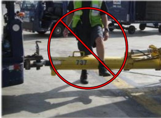
Figure 3: Do not cross over towbars.
