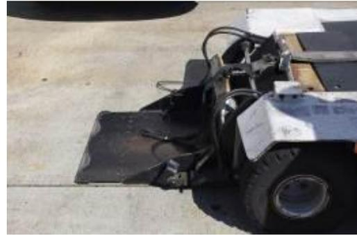
Figure 4: Lowered cradle on towbarless pushback
